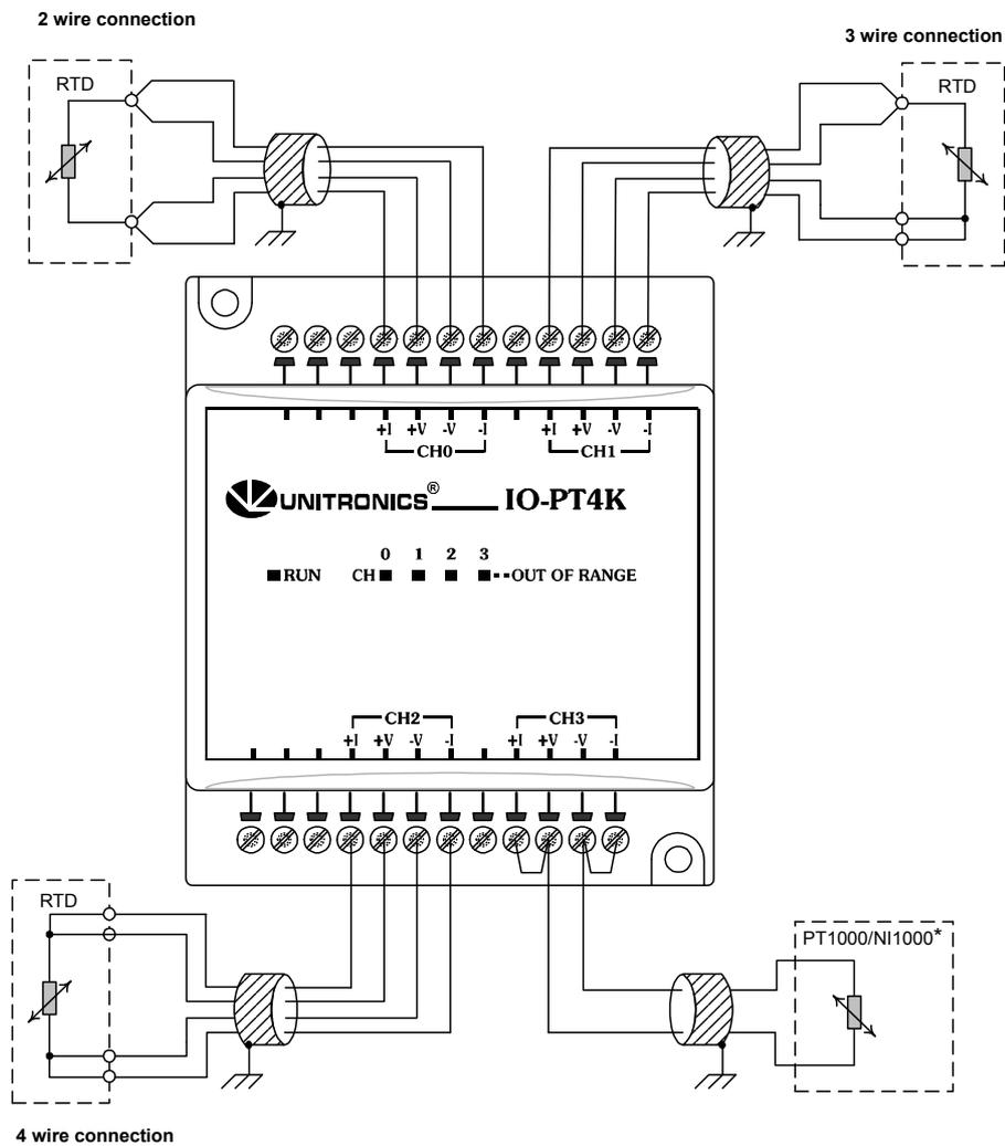
\* RTD input types PT1000/Ni1000 support a two-wire connection, because the high resistance (1000 ohm) of the sensor element compensates for voltage drop.
