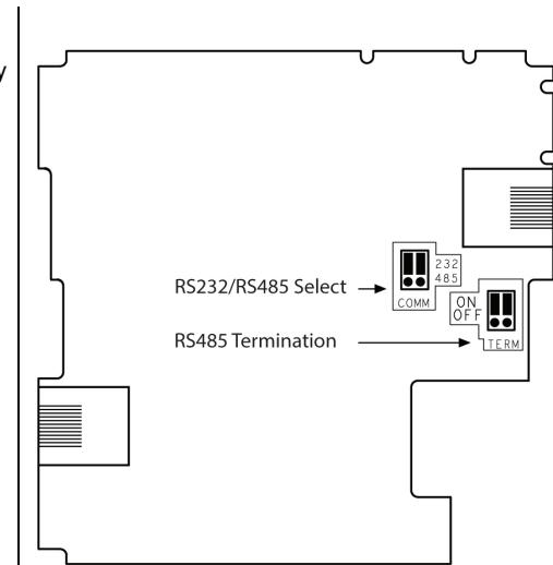
Note: it is possible to establish a PC to PLC connection using RS232 even when the PLC is set to RS485 (this will eliminate the need to open the controller for jumper setting). To do so, removes the RS485 connector (pins 1 & 6) from the PLC and connect a standard RS232 programming cable instead. Note that this is possible only if DTR and DSR signals of RS232 are not used (which is the standard case).
