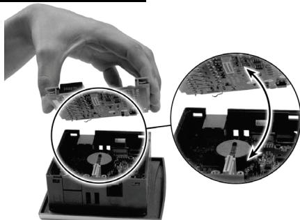
1. Gently replace the board. Make certain that the pins fit correctly into their matching receptacle. Do not force the board into place; doing so may damage the controller.
