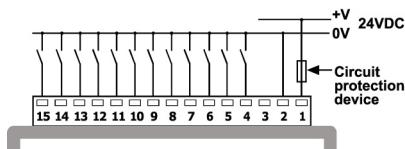
HSC input wiring, nPN (sink)
