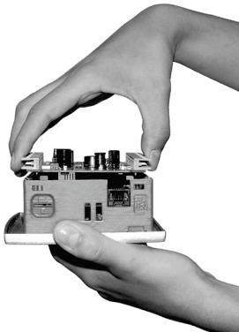
1. To access the communication jumpers, locate the screw close to COM port 1, and remove it.
