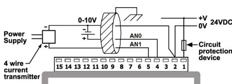
Analog input wiring, current (2/3 wire)
