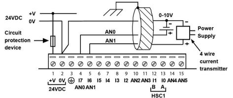
Shields should be connected at the signal's source.
