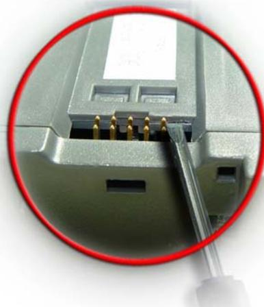
2. Taking care not to damage the cable, open the other side of the device by inserting the blade where shown below, then gently pushing up.
