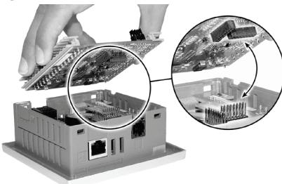
1. Gently replace the board. Make certain that the pins fit correctly into their matching receptacle. Do not force the board into place; doing so may damage the controller.
