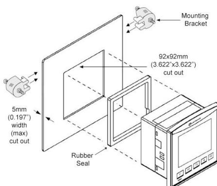
4. When properly mounted, the controller is squarely situated in the panel cut-out as shown in the figure to the right.
