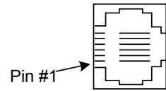
\*Standard programming cables do not provide connection points for pins 1 and 6.
