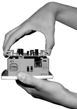
1. To access the communication jumpers, hold the I/O PCB board by its top and bottom connectors and steadily pull the board off.
