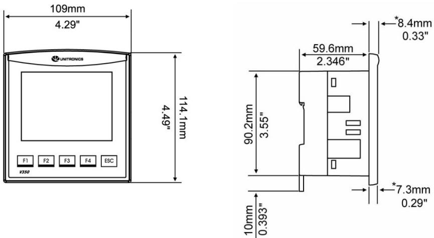
\* Note that for models V130J/V350J, the bezel width is 6.7 mm (0.26").
