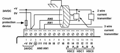
Analog input wiring, current (4-wire), voltage
