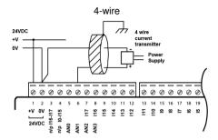
Analog Input wiring, voltage, (AN2-AN3)
