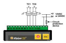
Shields should be connected at the signals' source.
